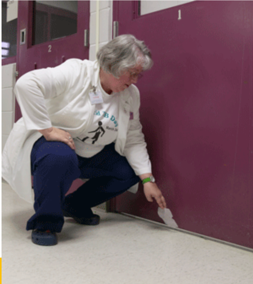
Checking negative pressure with a tissue
