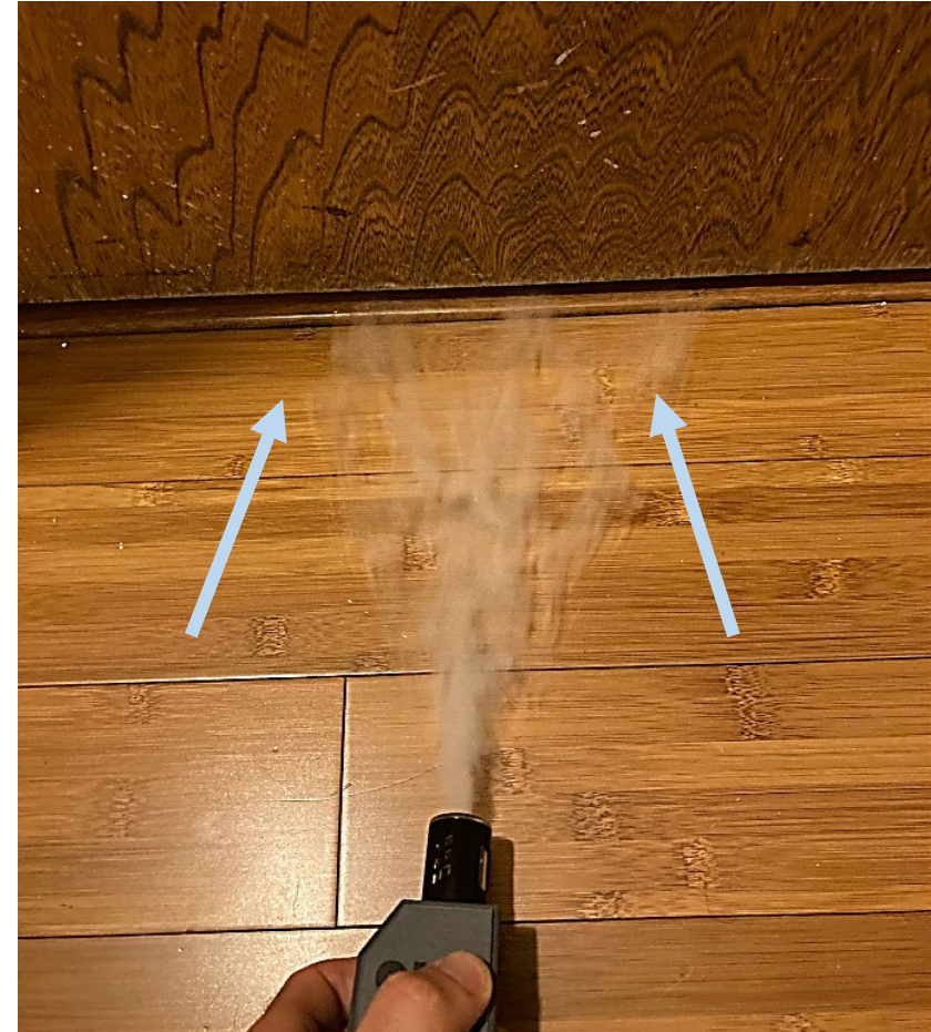
Non-toxic smoke following airflow into the room
