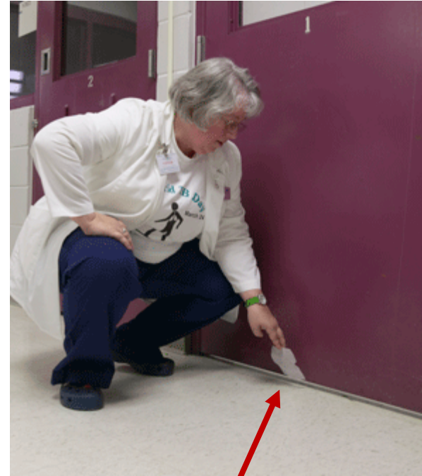
Tissue test: Place tissue outside door and see if it gets sucked into the room
